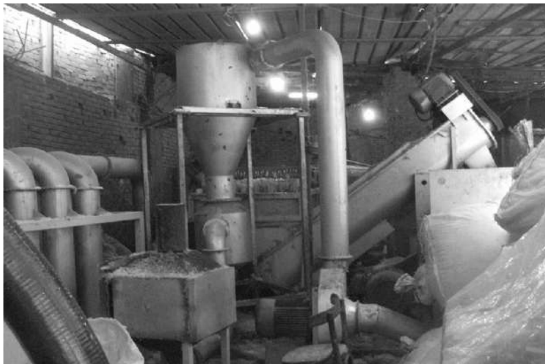
Figure 3. Automatic lines for crushing and cleaning plastic bags
